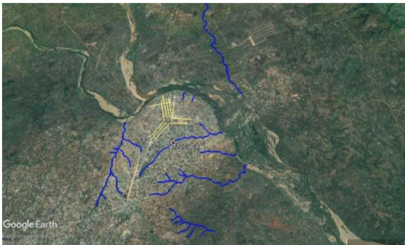
**FIGURA 40 PERCURSO DAS ÁGUAS SOB CANAIS DE DRENAGEM NATURAL**
